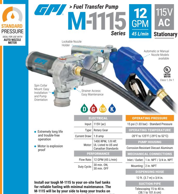
M-1115 will be by your side to keep your trucks on the road, your tractor working the fields, or your skid steer loader on the move until the job is finished.
