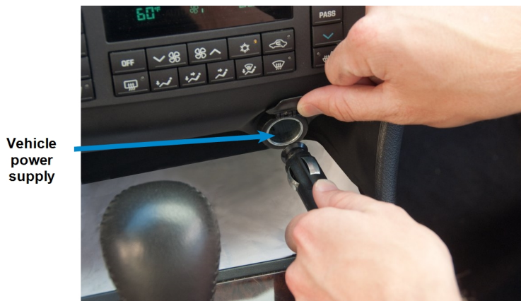
Figure 3.26 Vehicle Power Supply Cable Inserted in Car
