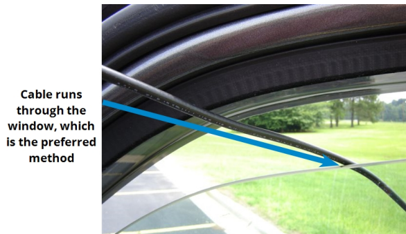
Figure 3.28 Antenna Cable Through Window
