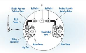
Manifolded systems provide up to 2X the flow rate and improved uptime. Manifolded systems can be configured in sumps 42" in diameter or greater.
