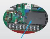
ISOTROL 1-8 may be ordered with or without the durable 30-amp power relay. Units without the relay are designed for use with another component for motor control. Units with the relay may "stade-alone" and will accept up to eight individual dispenser signals.
