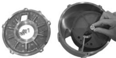
FIGURE 19 CHECKING THE PISTON MOVEMENT
