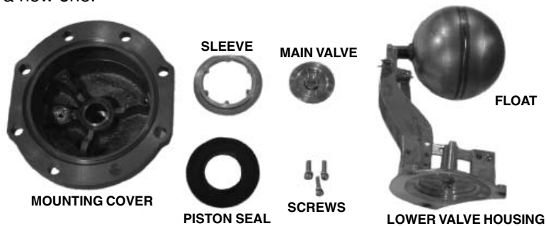
FIGURE 15 VAPOR/AIR RELEASE COMPONENTS
